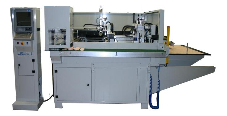
The cutting system "Saturno 2 Cutter" has been created to cut every type of material to sheets: fiberboard, reinforced thick up to 10 mm.
